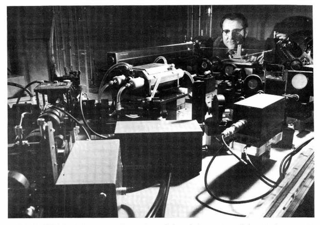
MURPHY LANDRY (1441) demonstrates his complex multiple cavity laser system which creates four separate beams from a single ruby rod in burst intervals as short as 20 nanoseconds. Art McCarthy (1441) and Henry Scheller (7651) assisted with the instrumentation of the laser system.
